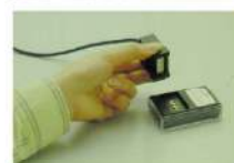
Use the probe checker to inspect probe connection.
