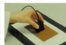
Put the probe perpendicular to the sample.
